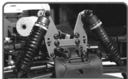
Long travel front suspension with increased up-travel. (Makes the car more forgiving and easier to drive)
