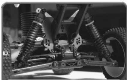
Long travel rear suspension with increased up-travel. (Makes the car more forgiving and easier to drive)
